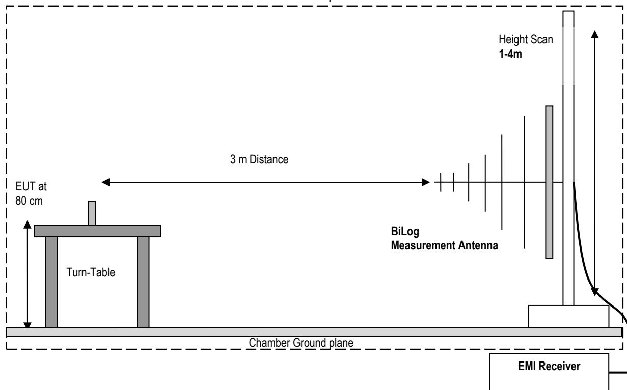
**Radiated Emissions Test Setup above 1GHz Measurements**
