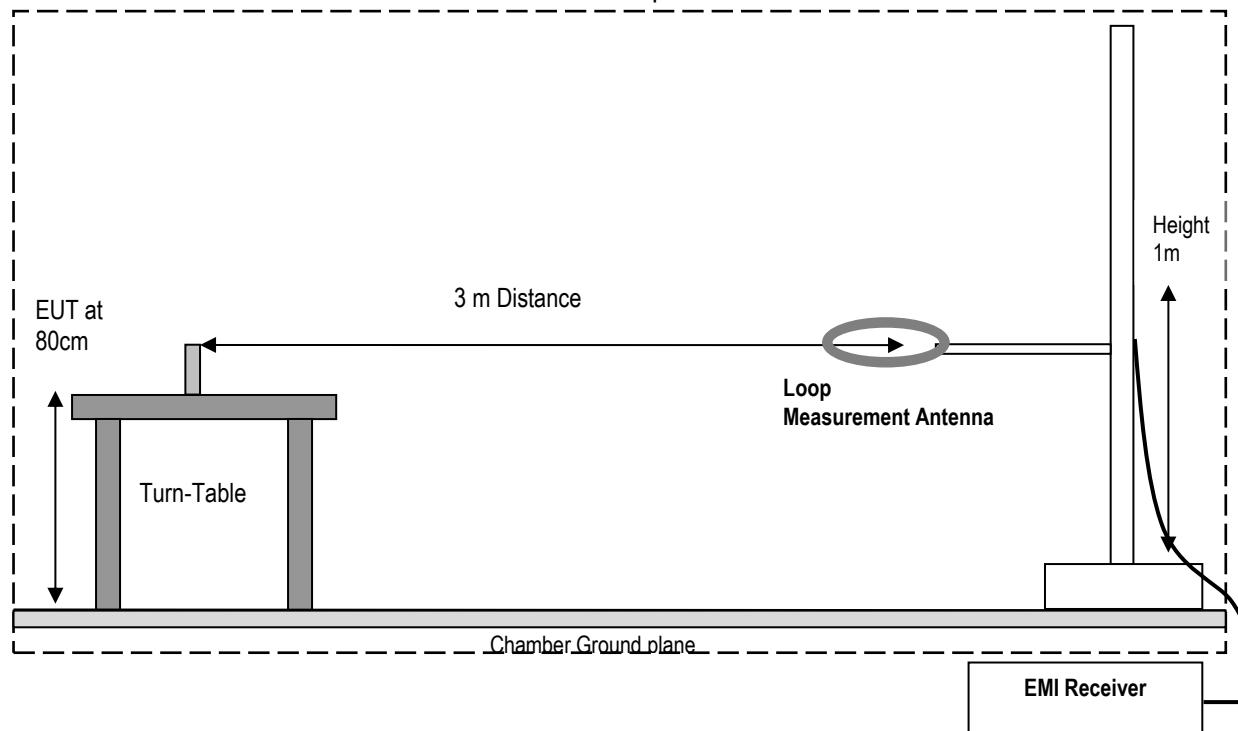
**Radiated Emissions Test Setup 30MHz-1GHz Measurements**
