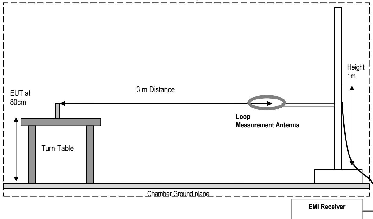
**Radiated Emissions Test Setup 30MHz-1GHz Measurements**
