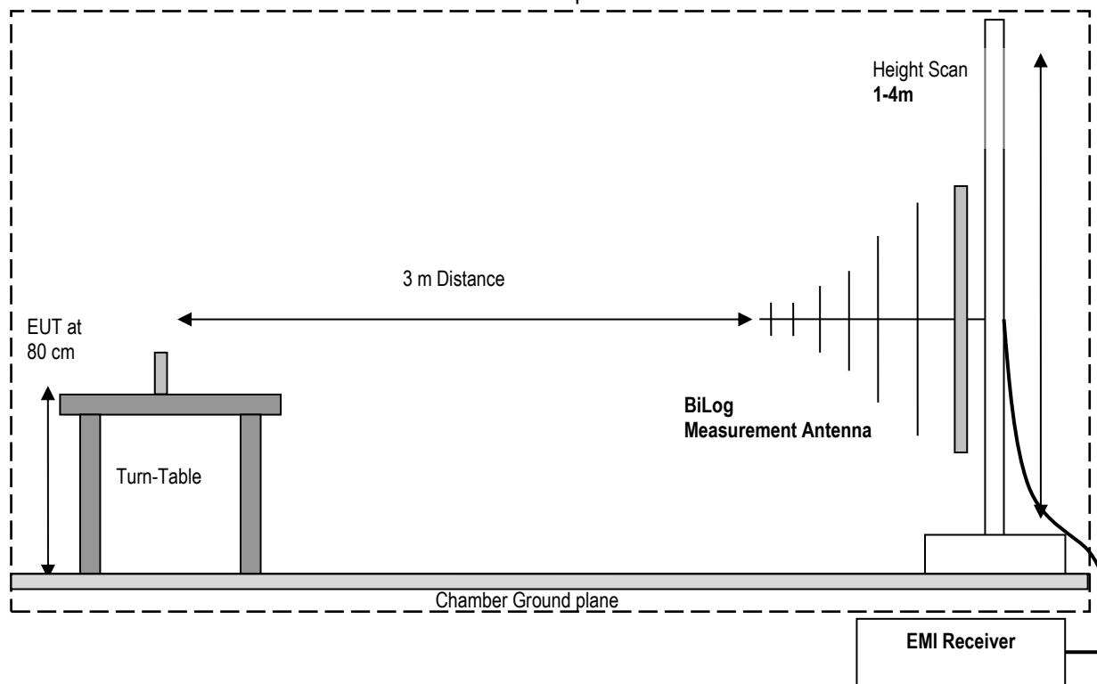
**Radiated Emissions Test Setup above 1GHz Measurements**
