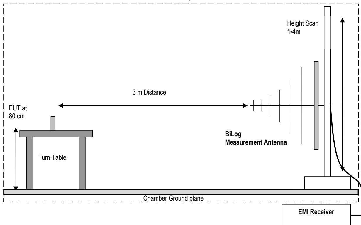
Radiated Emissions Test Setup above 1GHz Measurements
