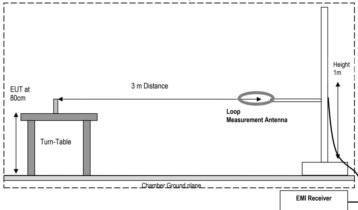
Radiated Emissions Test Setup 30MHz-1GHz Measurements
