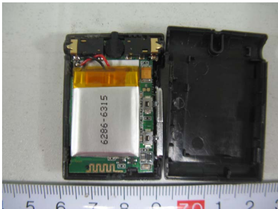
EUT - Main Board Top Components View
