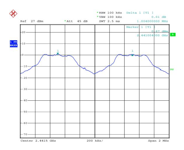
Xinwei M/N:T15s channel separation middle channel
