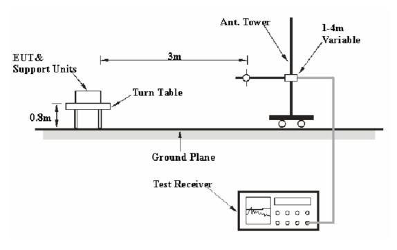
The radiated emission tests were performed in the 3 meters chamber B test site, using the setup accordance with the ANSI C63.4-2003. The specification used was the FCC 15.109, FCC 15.209 and FCC 15.247 limits.
