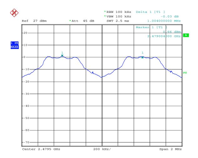
Xinwei M/N:T15s channel separation high channel
