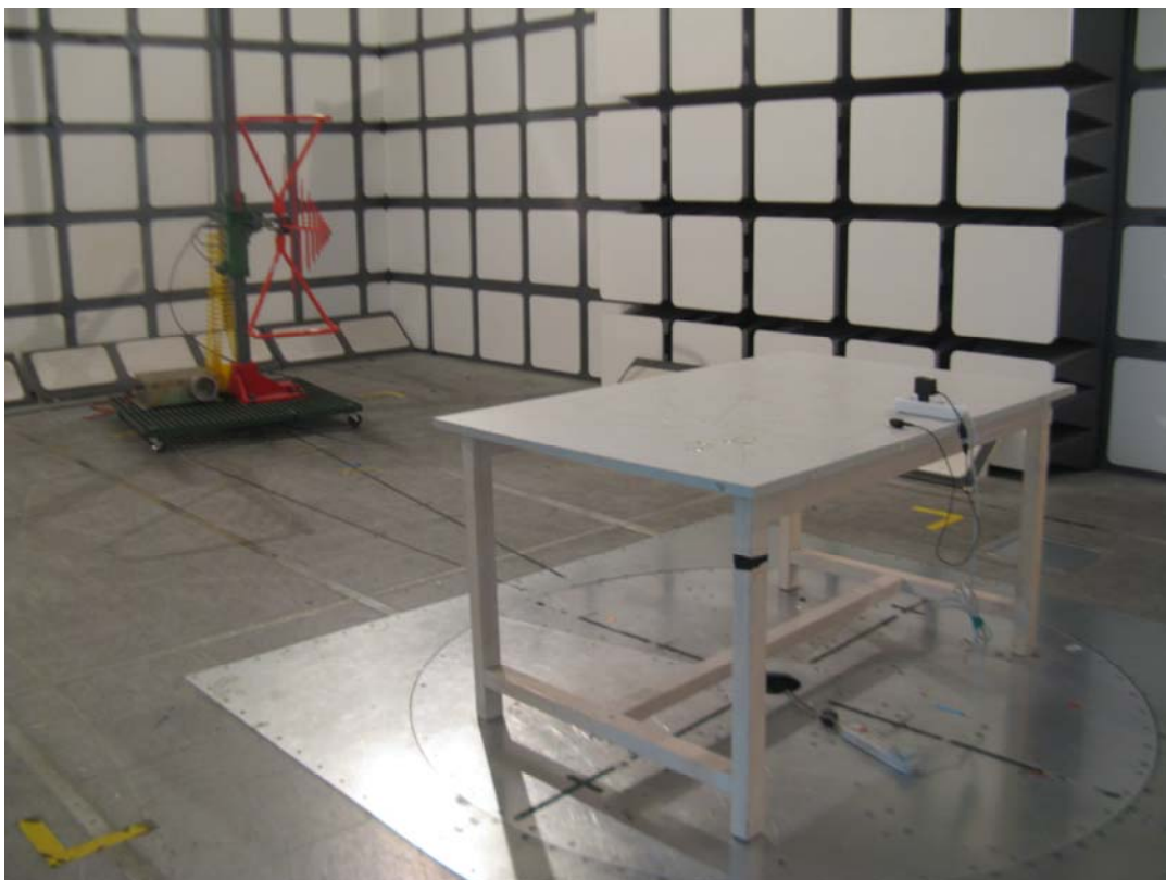
Charging Mode: Radiated Emissions - Rear View
