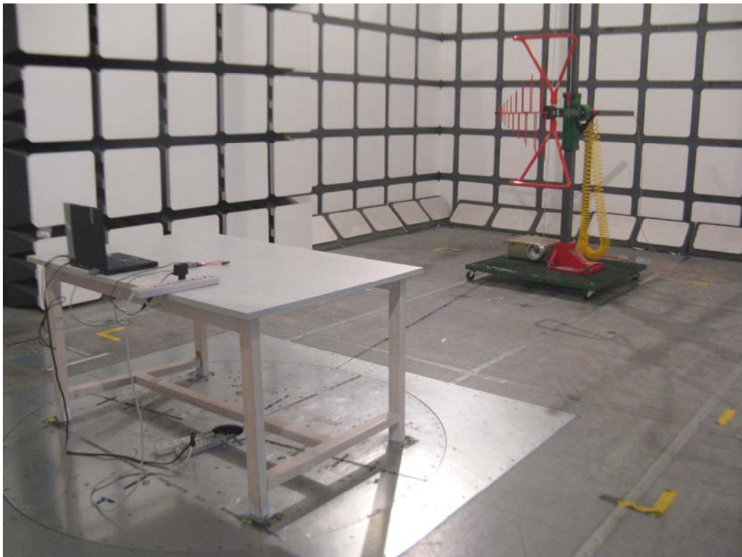
Transmitting Mode: Radiated Emissions - Rear View (30 MHz-1000MHz)
