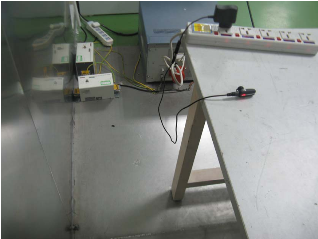
Charging Mode: Conducted Emissions - Side View
