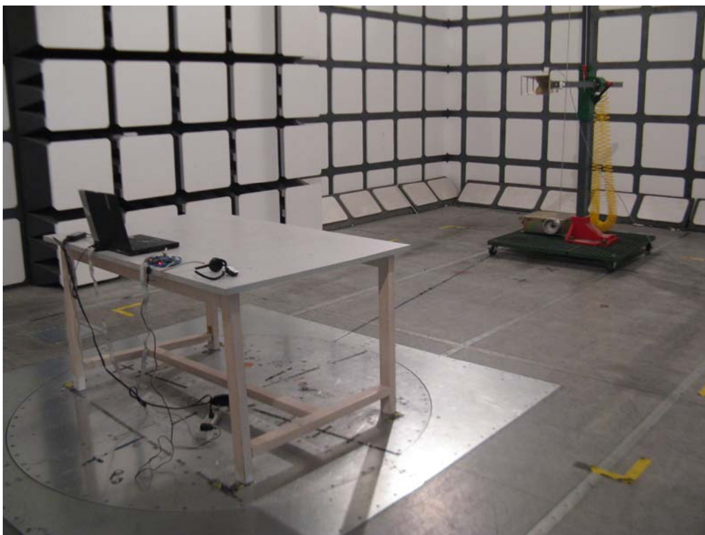
Transmitting Mode: Radiated Emissions - Rear View (Above 1 GHz)
