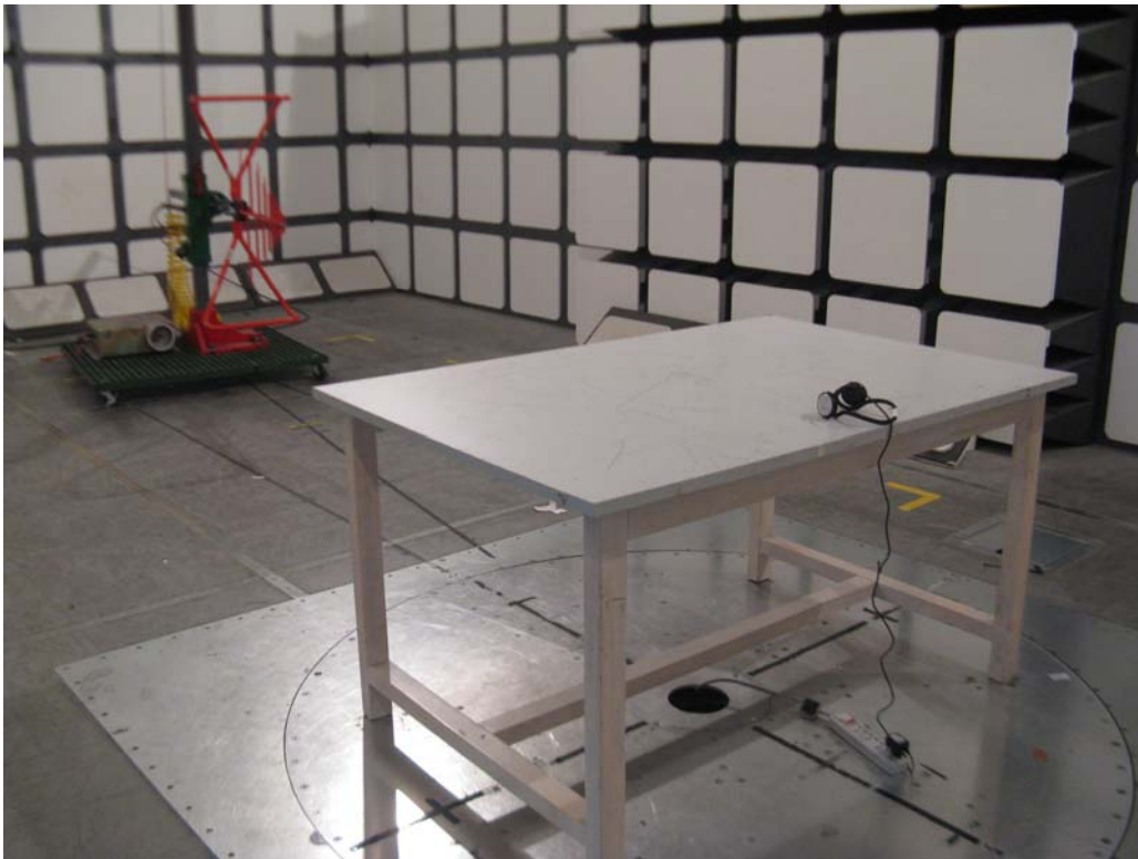
Charging Mode: Radiated Emissions - Rear View (30 – 1000 MHz)
