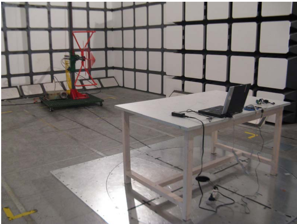
Transmitting Mode: Radiated Emissions - Rear View (30 – 1000 MHz)
