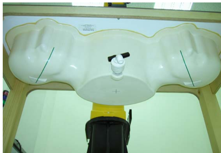
Fig. 5.4 Bottom view of twin phantom
