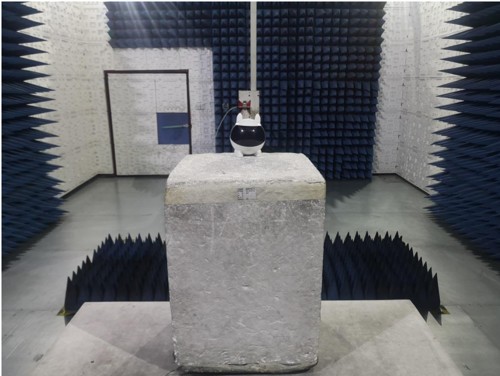
RADIATED EMISSION TEST SETUP ABOVE 1GHZ
