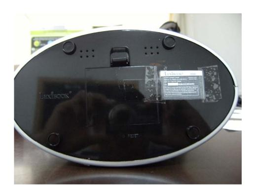
WB400\_09 Main station rating label size /dimension: 35 x 22 mm
