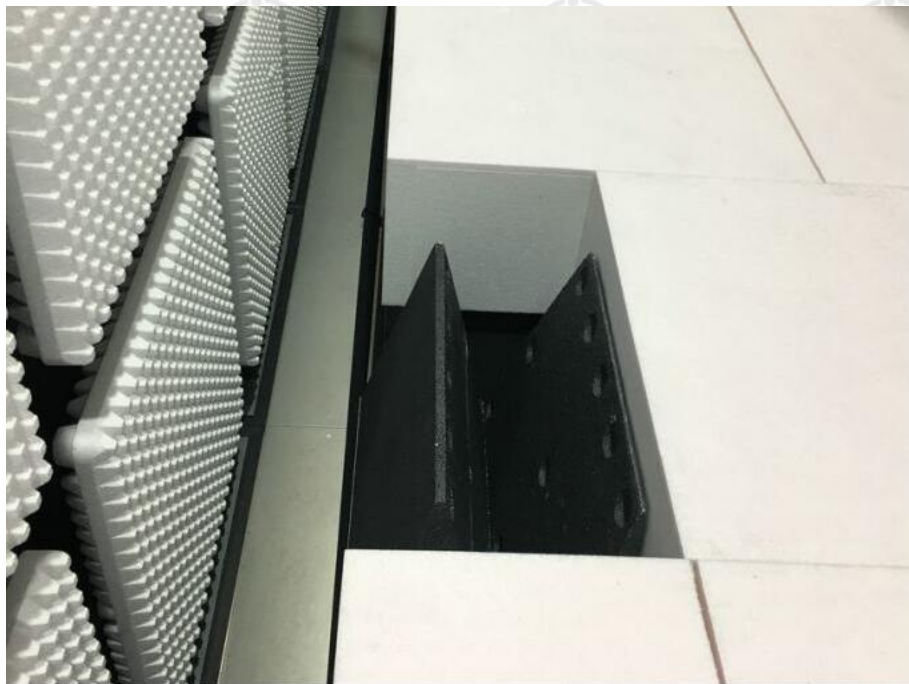
Radiated spurious emission Test Setup-4(Above 1GHz) There are absorbing materials under the ground.
