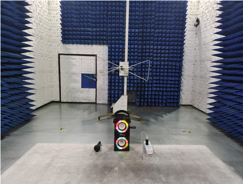
RADIATED EMISSION TEST SETUP ABOVE 1GHz
