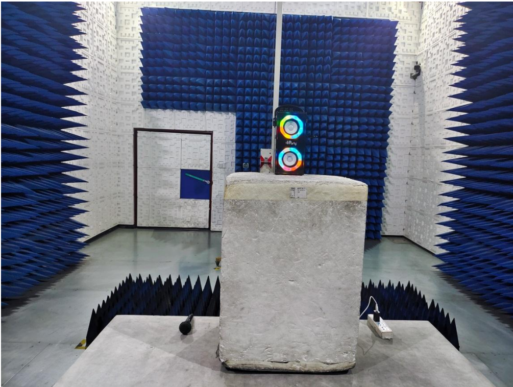
RADIATED EMISSION TEST SETUP ABOVE 1GHz
