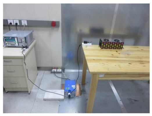
FCC RADIATED EMISSION TEST SETUP
