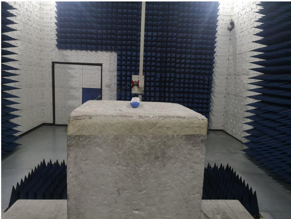
FCC RADIATED EMISSION TEST SETUP ABOVE 1GHZ
