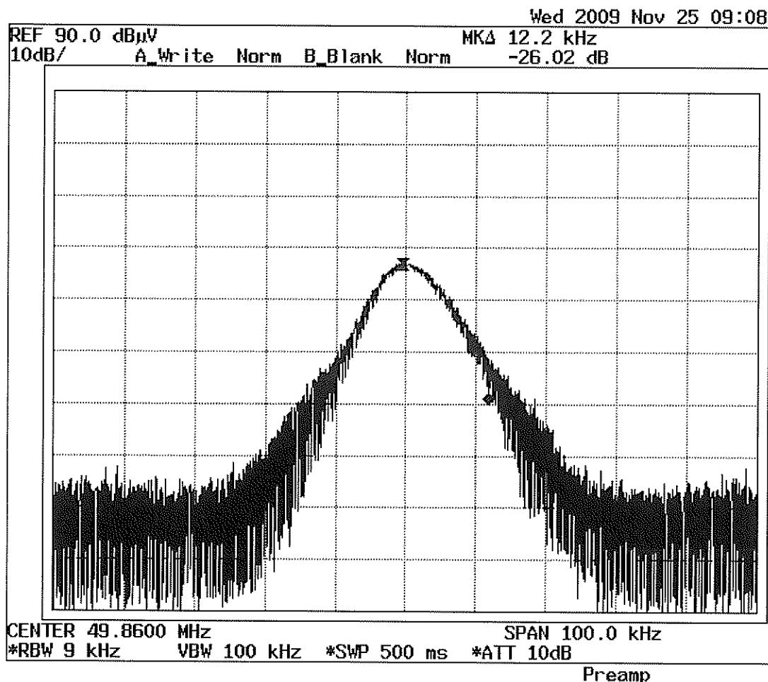
Result : The field strength of any emission within the operation band did not exceed 80 dB( $\mu$ V/m) for average value or 100 dB( $\mu$ V/m) for peak value. Refer to page 9 for the recorded value for the emission at the fundamental frequency.
