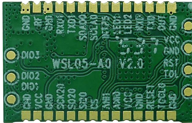
Figure 8-5 Bottom view of WSL05-A0 module
