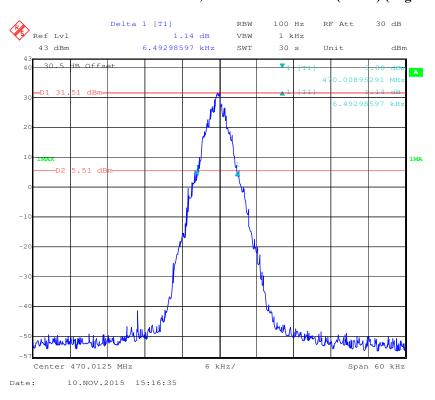
26 dB Emissions Bandwidth 12.5 kHz, 470.0125 MHz 4FSK (19200) (Low Power)
