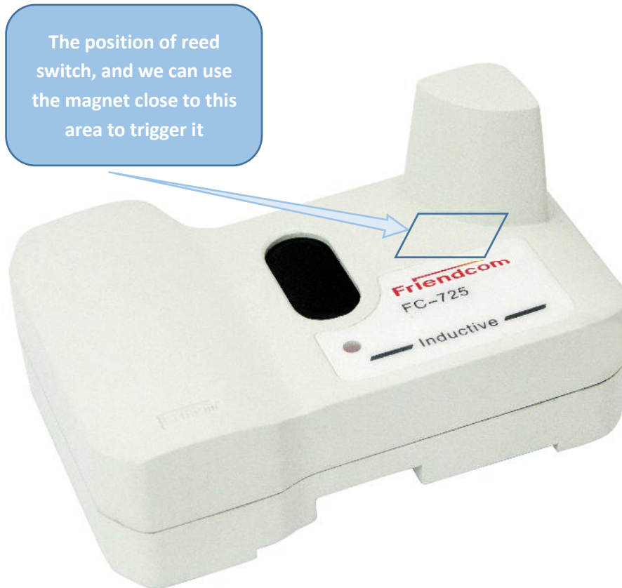
Figure 5-1 Magnet activation position
