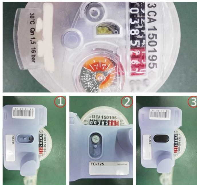
Figure 5-2 Installation of IDUV915-LRW
