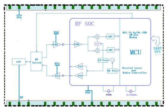
Note: The above block diagram is only used to indicate the internal structure of the module.
