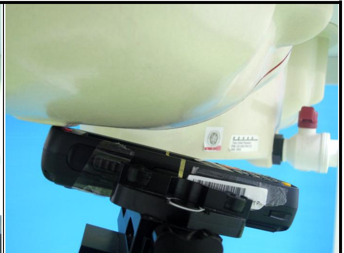
Right Tilted (EUT+Battery1)
