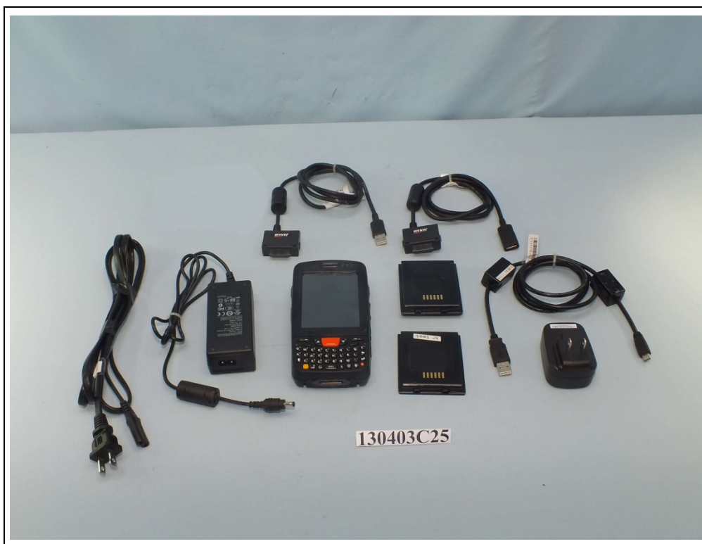
EUT with 1D barcode scanner
