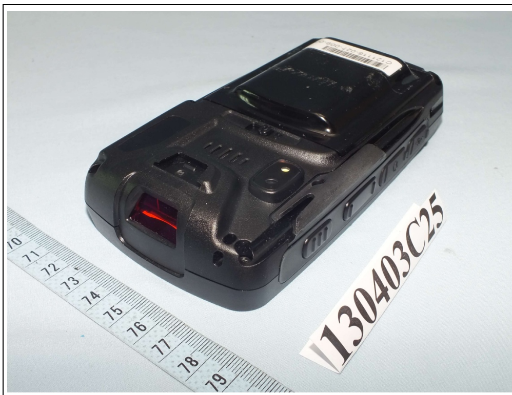
EUT with 2D barcode scanner
