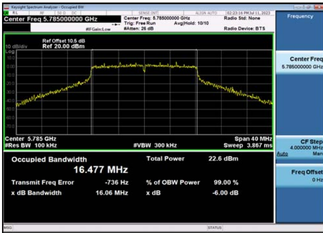
U-NII-3 6dB Bandwidth-802.11ac(20MHz) ,5745MHz,Ant1
