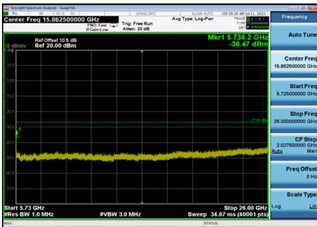
U-NII-2c ,Plot 1,Band Edge-802.11n(40 MHz),5550MHz,Ant1
