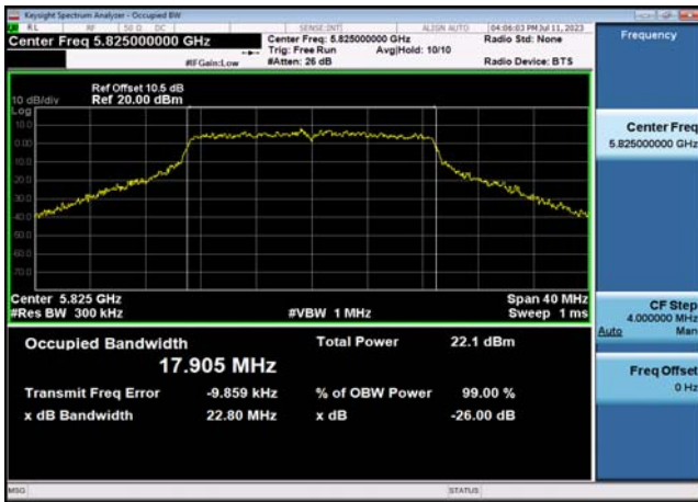
U-NII-3 99% Bandwidth-802.11ac(40MHz) ,5795MHz,Ant1
