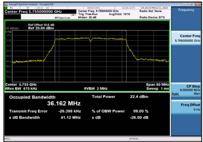
U-NII-3 99% Bandwidth-802.11ac(80MHz) ,5775MHz,Ant1
