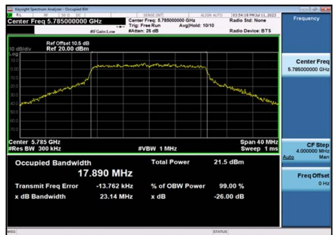
U-NII-3 99% Bandwidth-802.11ac(20MHz) ,5785MHz,Ant1
