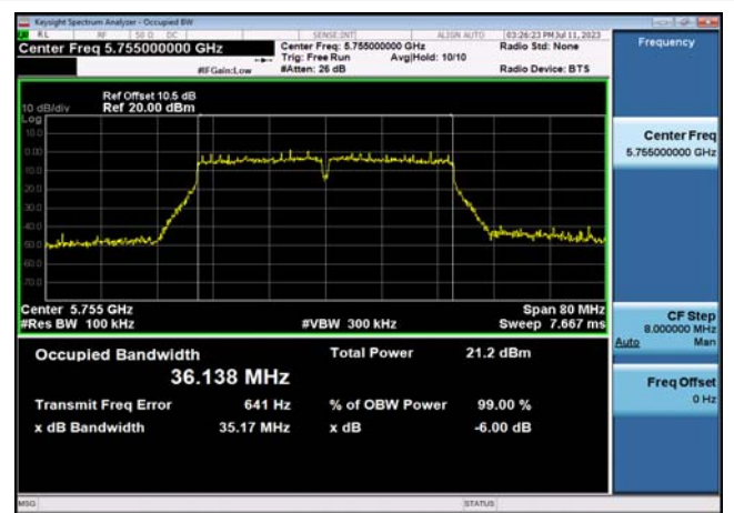
U-NII-3 6dB Bandwidth-802.11a(20MHz) ,5745MHz,Ant1
