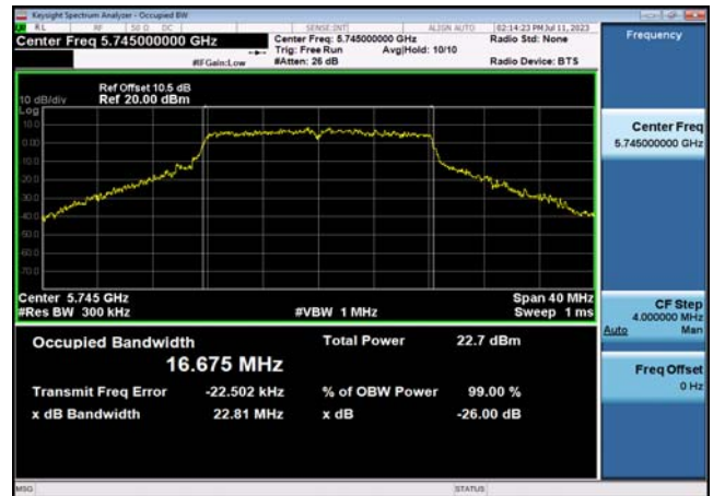
U-NII-3 99% Bandwidth-802.11a(20MHz) ,5825MHz,Ant1
