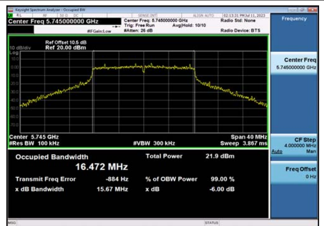
U-NII-3 6dB Bandwidth-802.11a(20MHz) ,5745MHz,Ant1
