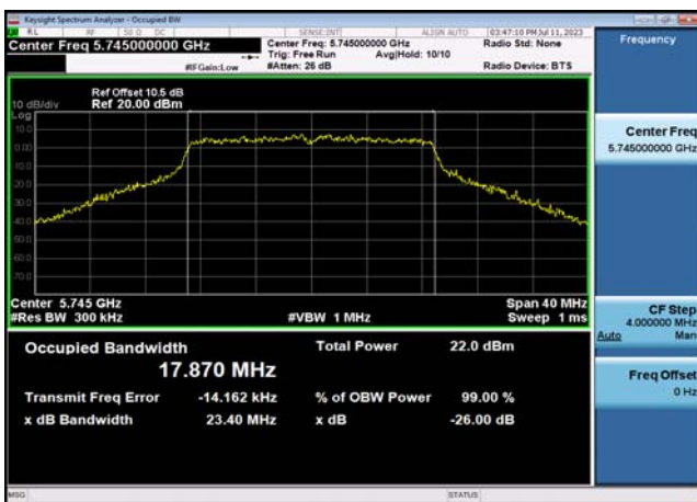
U-NII-3 99% Bandwidth-802.11ac(20MHz) ,5745MHz,Ant1
