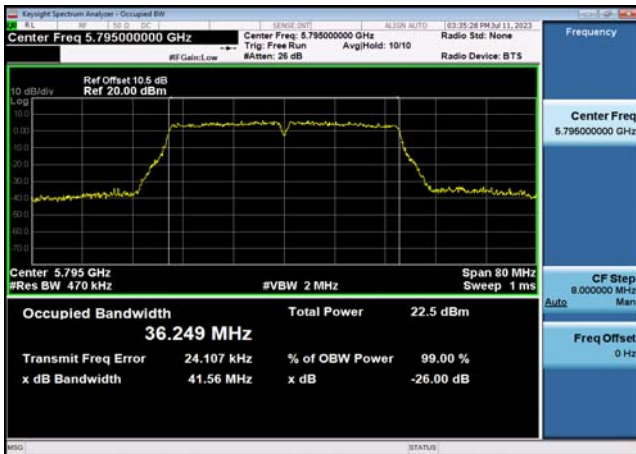
U-NII-3 99% Bandwidth-802.11a(20MHz) ,5785MHz,Ant1
