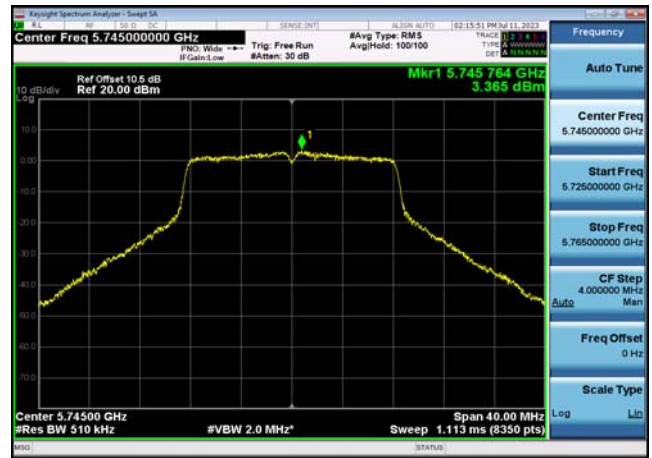
U-NII-3 Power spectral density-802.11 a(20MHz),5825MHz,Ant1
