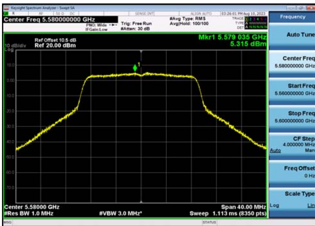
U-NII-2c Power spectral density-802.1 1ac(40MHz),5510MHz,Ant1
