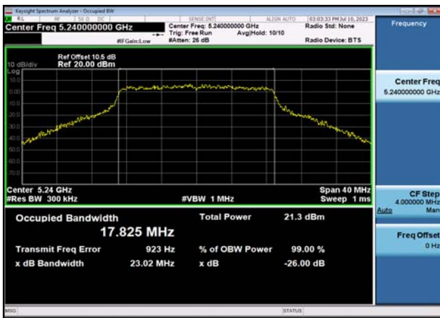
U-NII-1 26dB&99% Bandwidth-802.11ac(20MHz) ,5240MHz,Ant1
