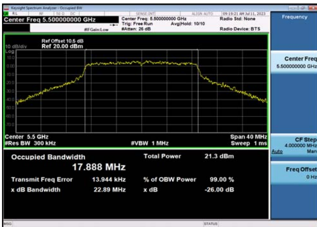
U-NII-2c 26dB&99% Bandwidth-802.11n(20MHz),5500MHz,Ant1
