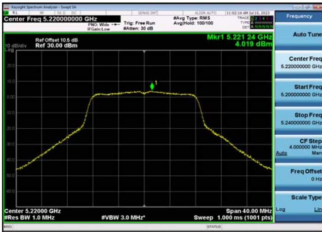
U-NII-1 Power spectral density-802.11 ac(20MHz),5180MHz,Ant1
