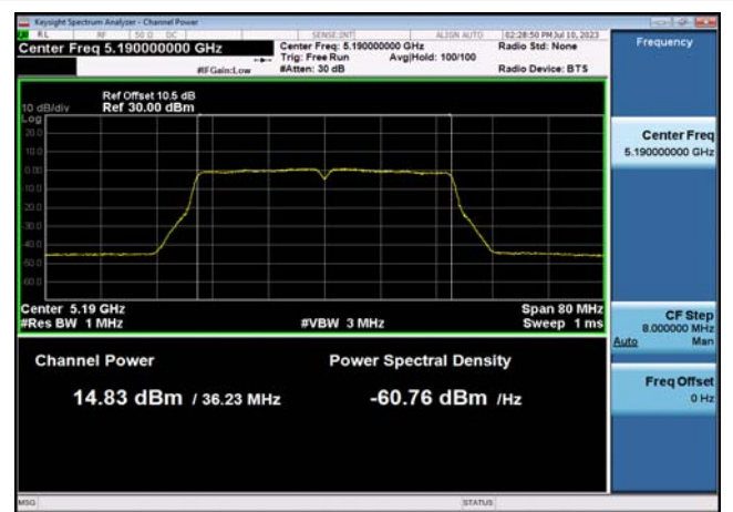
U-NII-1 Output Power-802.11a(20MHz) ,5180MHz,Ant1
