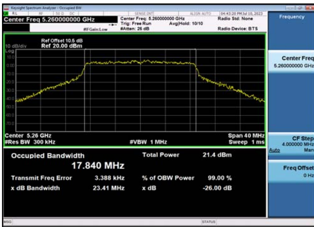
U-NII-2a 26dB&99% Bandwidth-802.11ac(20MHz) ,5260MHz,Ant1
