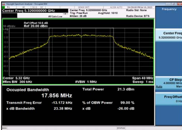
U-NII-2a 26dB&99% Bandwidth-802.11ac(40MHz),5310MHz,Ant1
