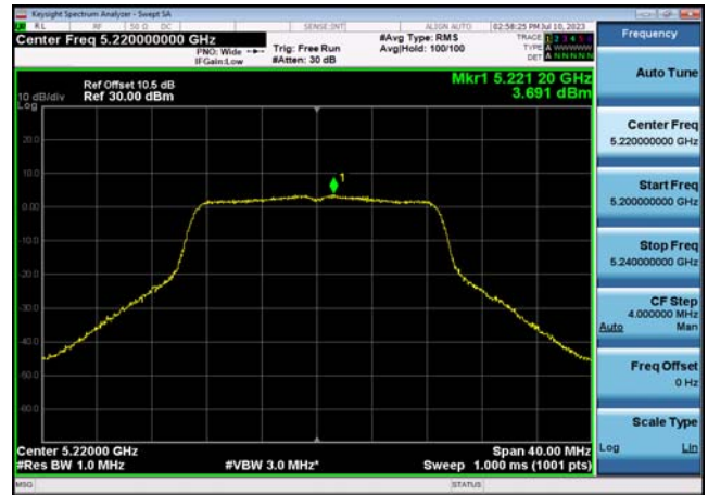
U-NII-1 Power spectral density-802.11 ac(40MHz),5190MHz,Ant1
