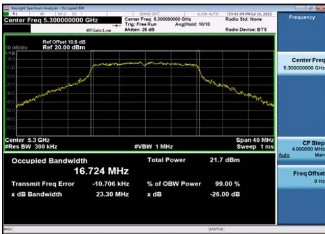
U-NII-2a 26dB&99% Bandwidth-802.11ac(20MHz) ,5260MHz,Ant1
