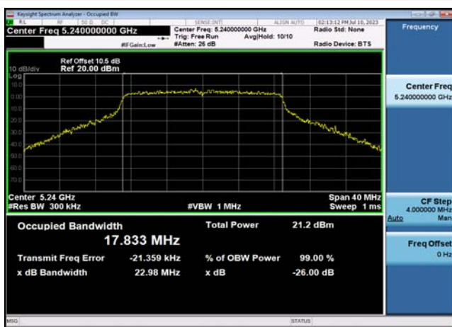
U-NII-1 26dB&99% Bandwidth-802.11n(40MHz) ,5230MHz,Ant1
