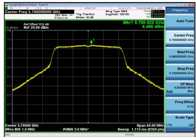
U-NII-2c Power spectral density-802.1 1ac(40MHz),5550MHz,Ant1
