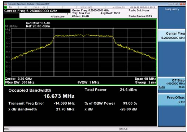
U-NII-2a 26dB&99% Bandwidth-802.11a(20MHz) ,5320MHz,Ant1
