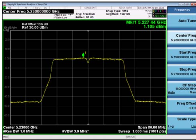
U-NII-2a Power spectral density-802.1 1n(20MHz),5260MHz,Ant1
