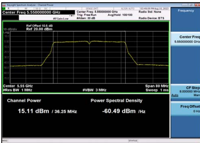
U-NII-2c Output Power-802.11a(20MHz) ,5500MHz,Ant1
