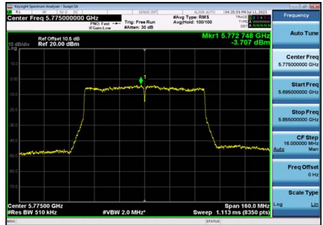
U-NII-3 Power spectral density-802.11 ac(80MHz),5775MHz,Ant1
