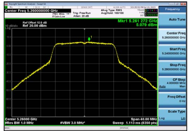
U-NII-2a Power spectral density-802.1 1a(20MHz),5320MHz,Ant1
