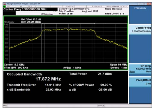
U-NII-2a 26dB&99% Bandwidth-802.11n(40MHz) ,5270MHz,Ant1
