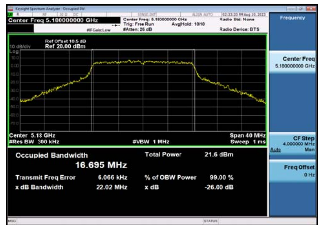
U-NII-1 26dB&99% Bandwidth-802.11a(20MHz) ,5180MHz,Ant1
