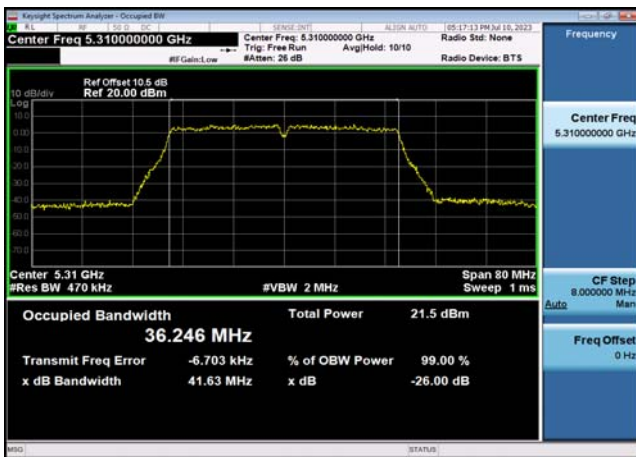
U-NII-2c 26dB&99% Bandwidth-802.11n(20MHz),5500MHz,Ant1
