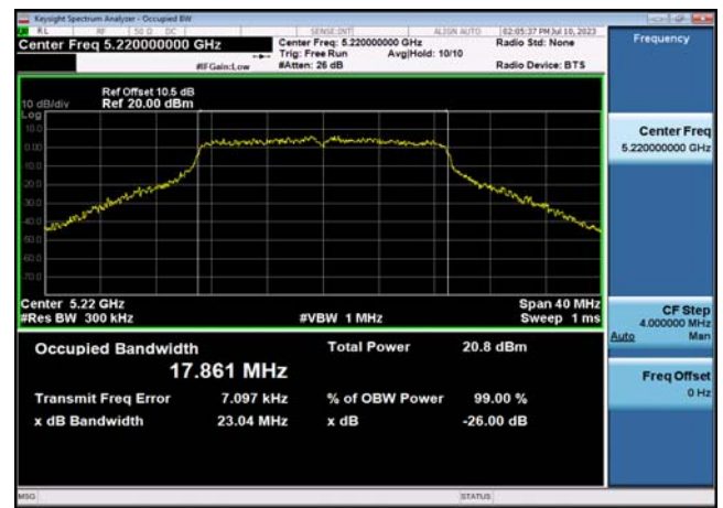
U-NII-1 26dB&99% Bandwidth-802.11n(40MHz) ,5190MHz,Ant1
