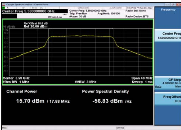
U-NII-2c Output Power-802.11ac(40MHz) ,5510MHz,Ant1
