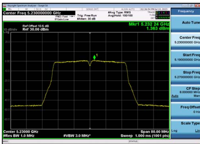
U-NII-1 Power spectral density-802.11 n(40MHz),5230MHz,Ant1
