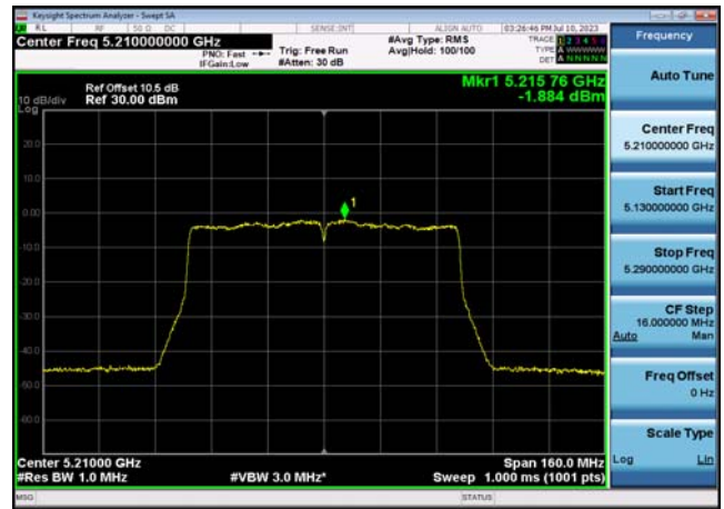
U-NII-2a Power spectral density-802.1 1n(20MHz),5300MHz,Ant1
