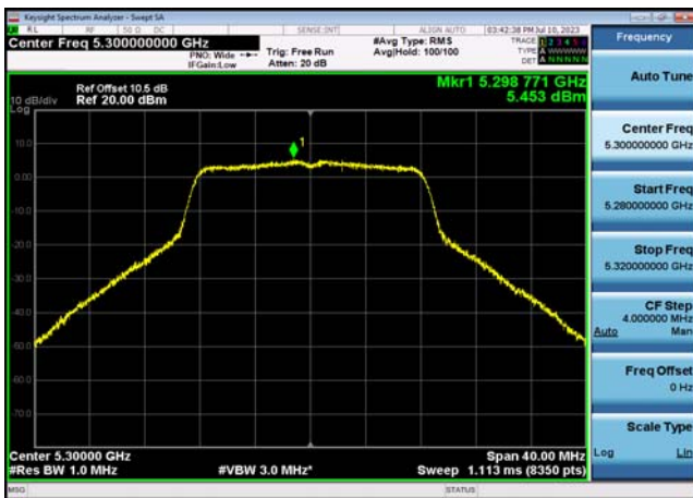
U-NII-2a Power spectral density-802.1 1ac(20MHz),5260MHz,Ant1
