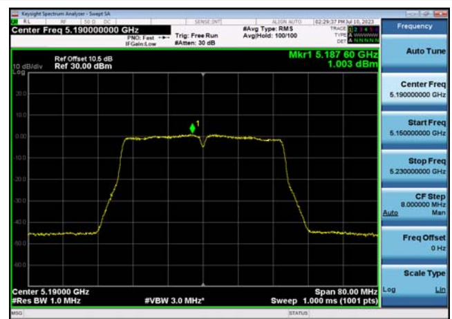
U-NII-1 Power spectral density-802.11 a(20MHz),5180MHz,Ant1
