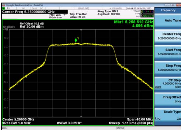
U-NII-2a Power spectral density-802.1 1ac(20MHz),5260MHz,Ant1
