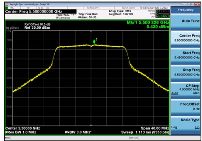
U-NII-2c Power spectral density-802.1 1ac(20MHz),5700MHz,Ant1
