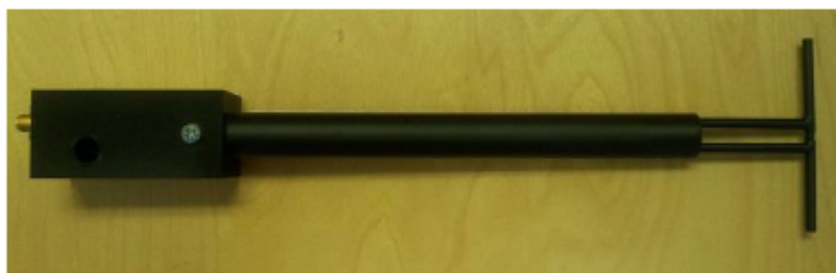
Figure 1 – MVG COMOSAR Validation Dipole
