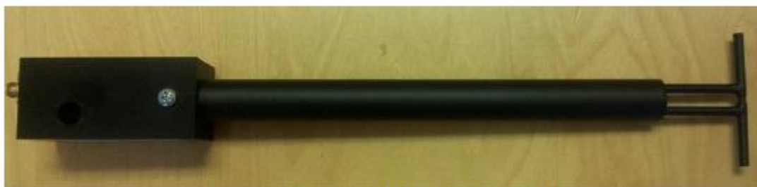
Figure 1 – MVG COMOSAR Validation Dipole
