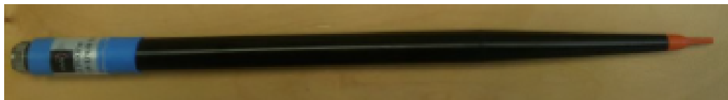
Figure 1 – MVG COMOSAR Dosimetric E field Dipole
