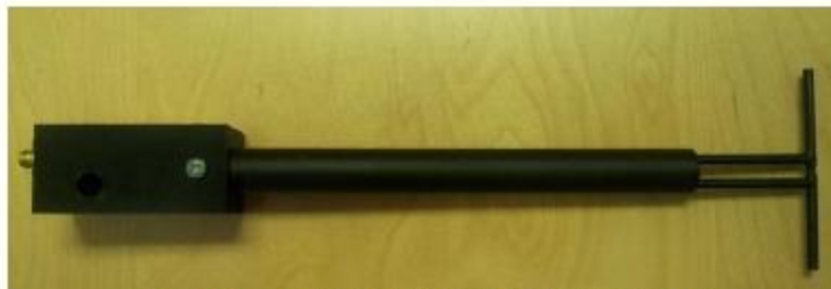
Figure 1 – MVG COMOSAR Validation Dipole
