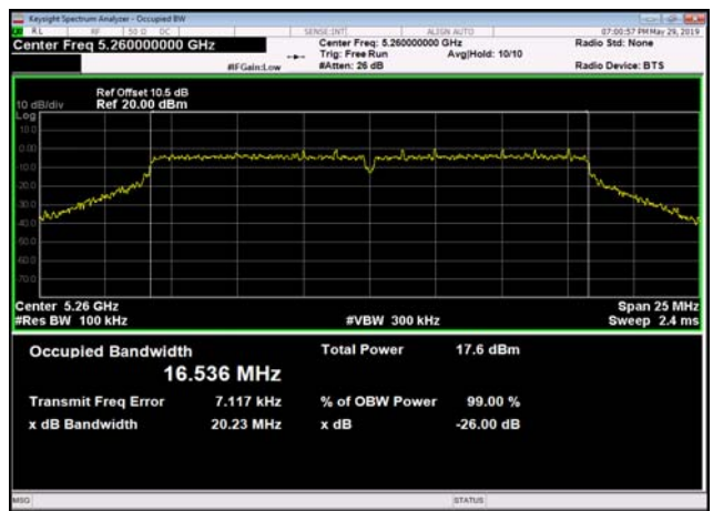
U-NII-2a 26dB Bandwidth-802.11a(20MHz) ,5260MHz
