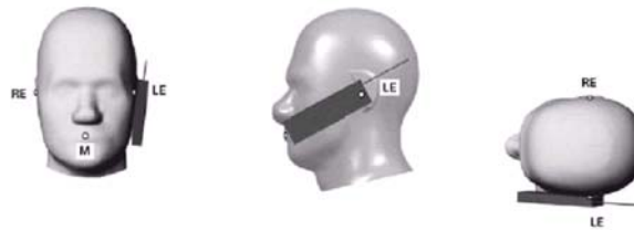
Figure 5.1 Front, Side and Top View of Cheek/Touch Position
