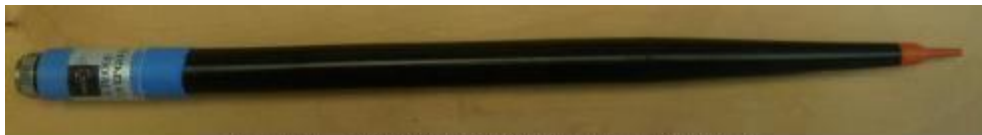
Figure 1 – MVG COMOSAR Dosimetric E field Dipole
