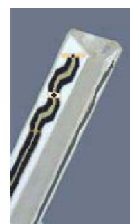
Figure 3.3 Probe Thick-Film Technique
