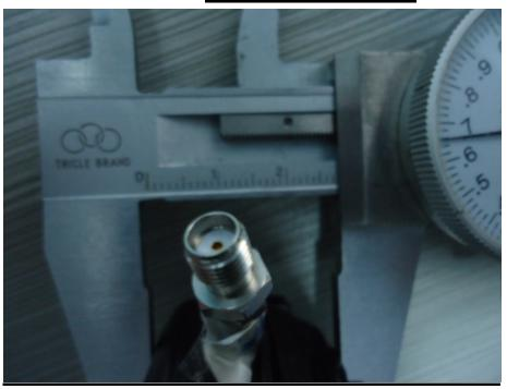
The thickness of EUT is about 28mm, The chip antenna is assembled on the PCB, The main PCB is assembled on the middle of the EUT, So the separation distances are about 14mm.
