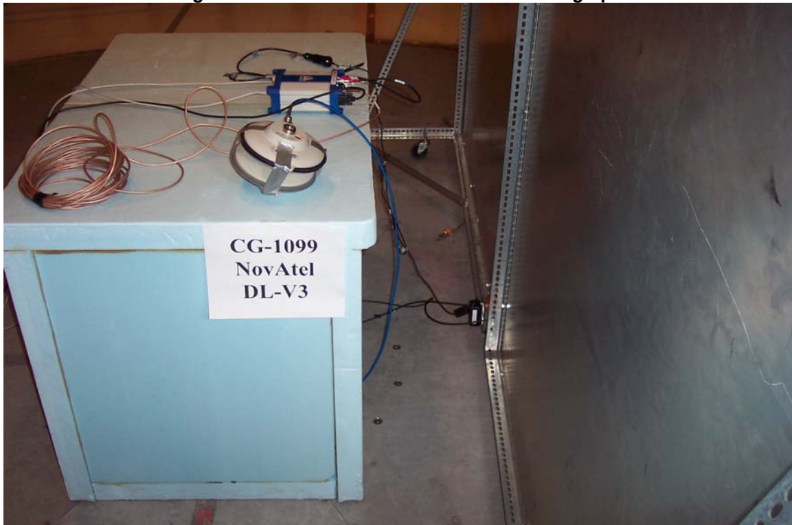
Figure 2 Conducted Emissions Test Photograph
