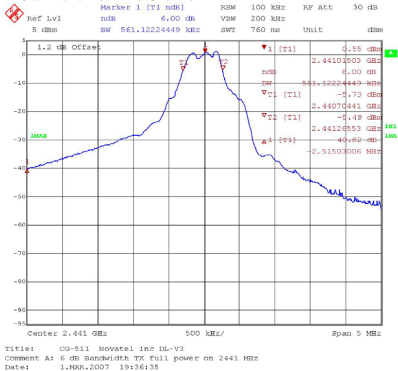
Figure 3 6 dB Bandwidth Upper Channel
