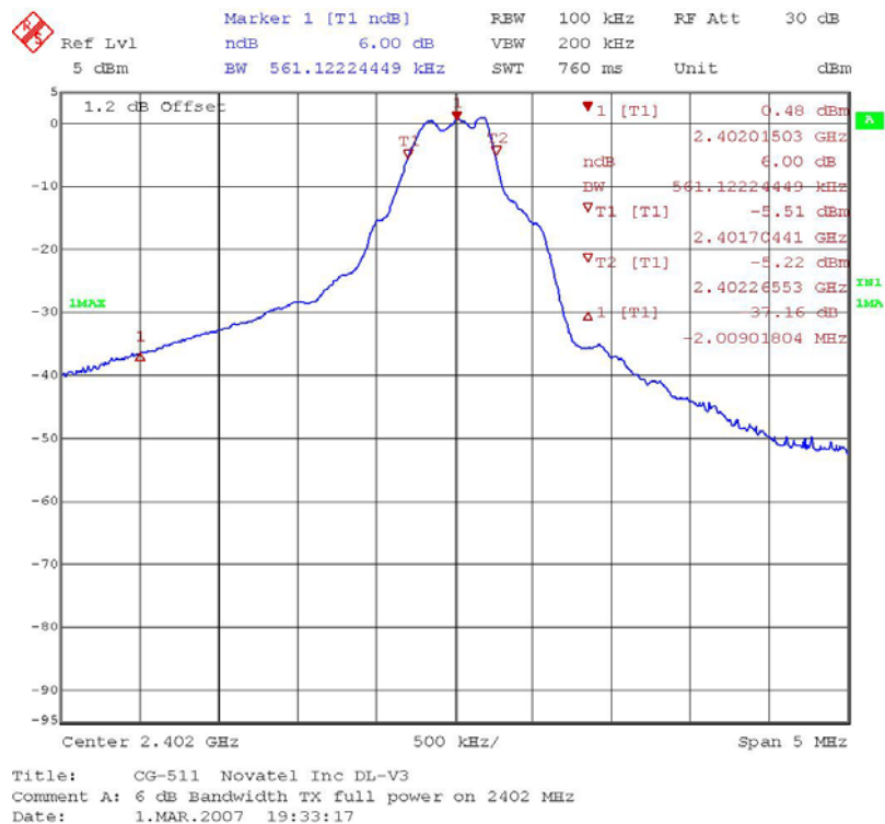
Figure 1 6 dB Bandwidth Low Channel
