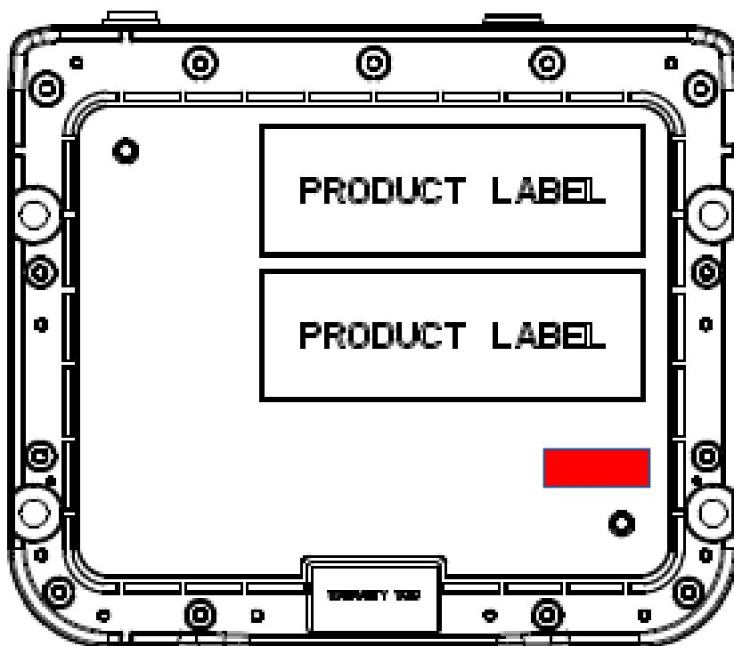
The FCC/ISED Identification is printed into the main product label at the location indicated by the **highlighted area**.
