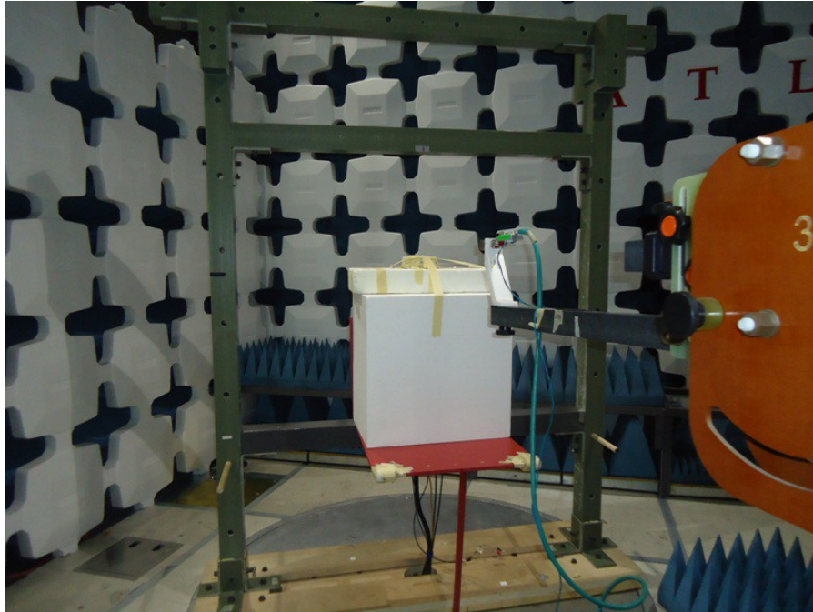
Figure 4.8 - Radiated Emission Test Setup - Front View
