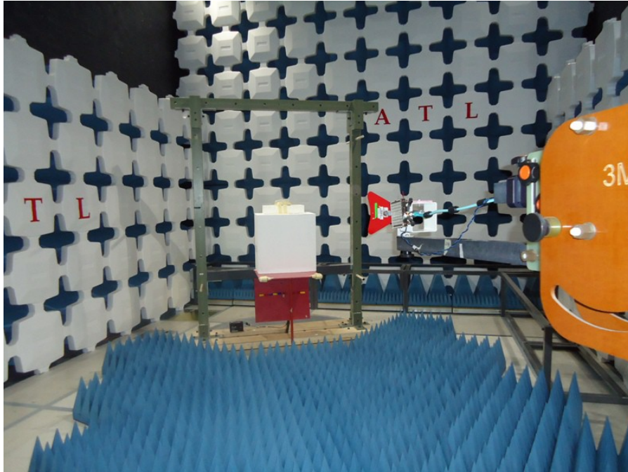
Figure 4.6 - Radiated Emission Test Setup - Front View
