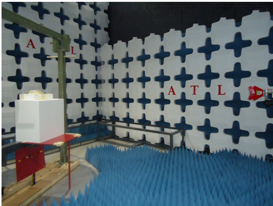
Figure 4.7 - Radiated Emission Test Setup - Side View
