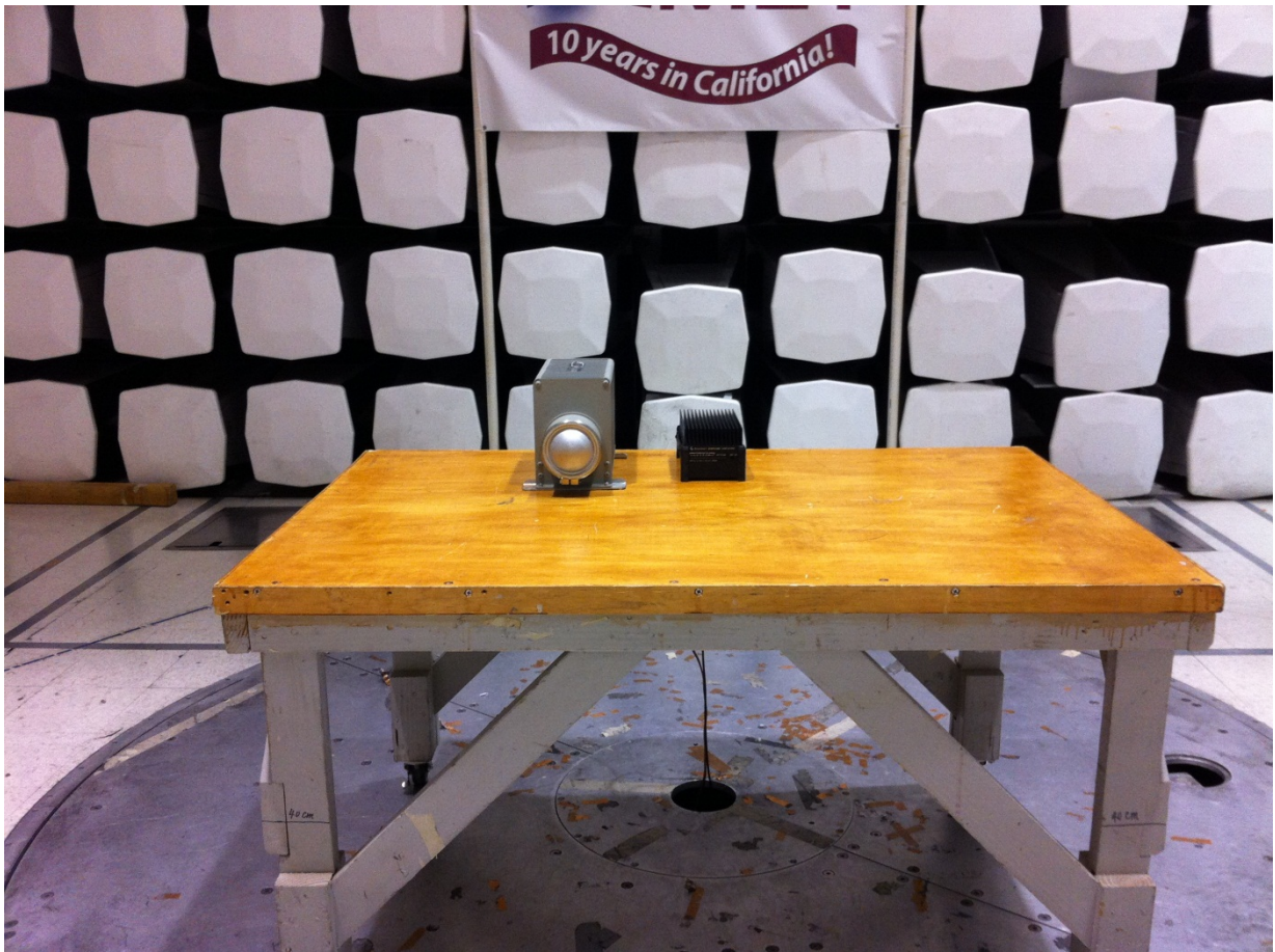
Photograph 7. 97.307(d) Radiated Spurious Emissions for TX Operating Below 30 MHz Test Setup (Front View)
