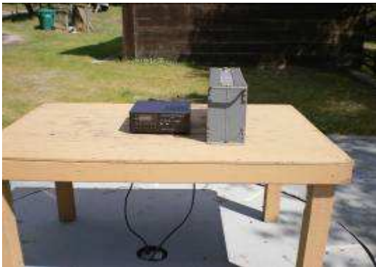
Unit under test with dummy load
