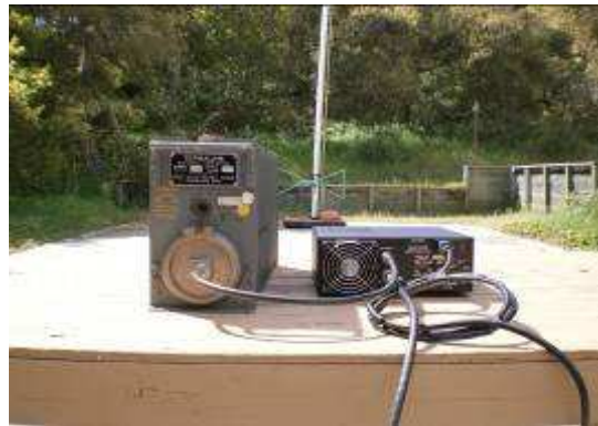
Unit under test with dummy load
