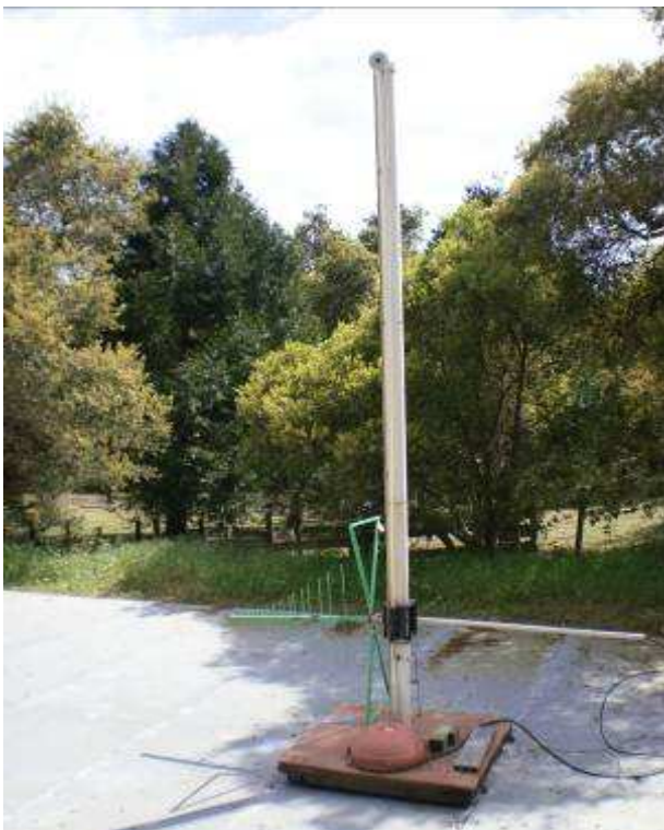
6141 receive antenna on height-adjustable pole
