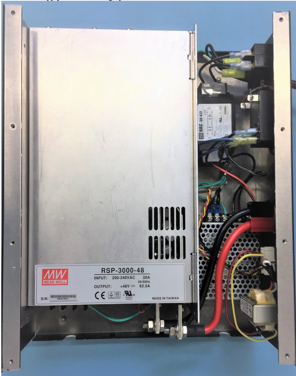
KPA1500 Power Supply Internal Photograph
