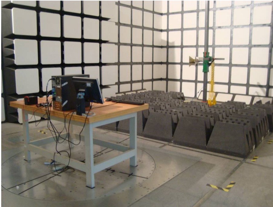
Above 1GHz: Spurious Radiated Emissions - Front View
