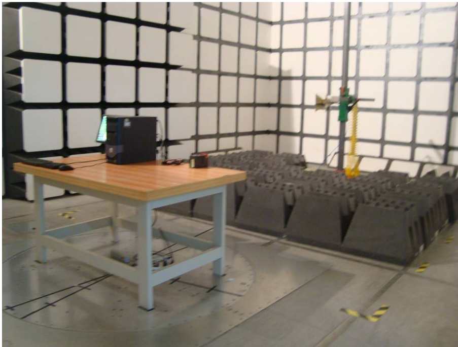
Above 1GHz: Spurious Radiated Emissions - Rear View
