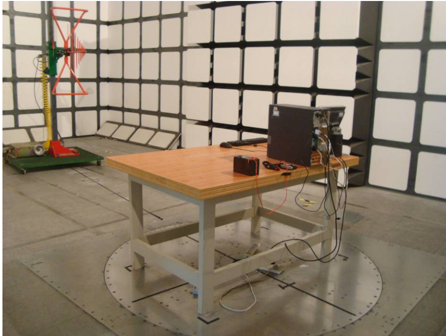
Below 1GHz: Spurious Radiated Emissions - Front View
