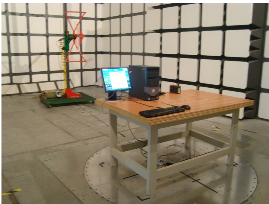
Below 1GHz: Spurious Radiated Emissions - Rear View
