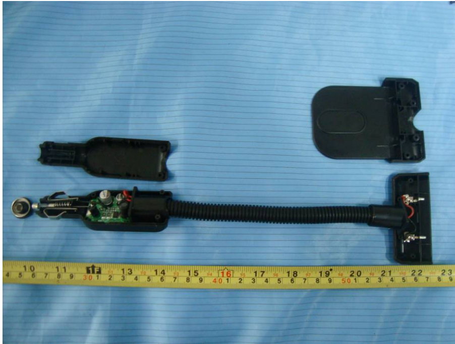
EUT – In-car Charger Cover off View
