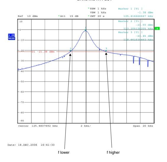
f lower = 123.205 kHz f higher = 128.462 kHz Occupied Bandwidth = 5.257 kHz
