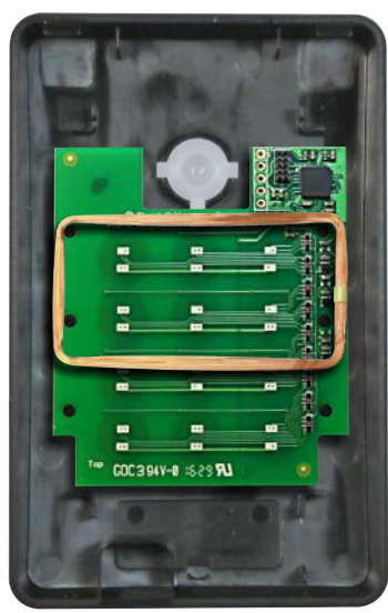
VIEW - REVERSE ▲ internal view part assembled LIGHTGUIDE + KEYPAD PCB + ANTENNA (reader unpotted)
