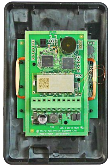
VIEW - REVERSE - internal view assembled + PCB top view (reader unpotted) ▲
