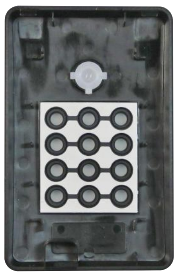
VIEW - REVERSE ▲ internal view part assembled LIGHTGUIDE + KEYPAD (reader unpotted)
