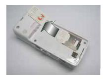
When you need to remove the SIM card, you should first switch off the phone, remove the battery, and take it away from under the SIM cardholder.
