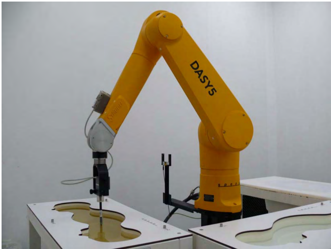
Picture 1: Specific Absorption Rate Test Layout
