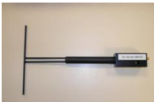
Figure 1 – Satimo COMOSAR Validation Dipole
