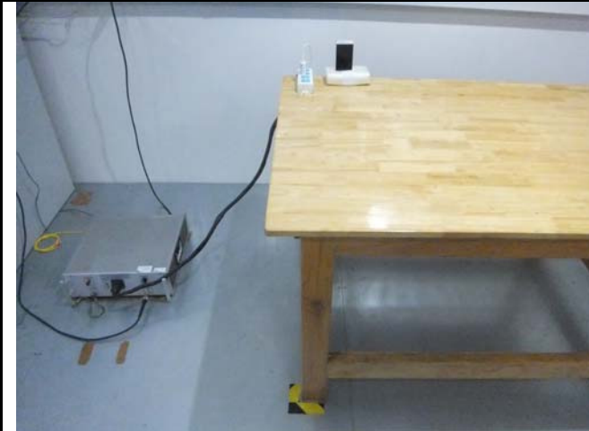
Conducted Emissions Test Setup Front View
