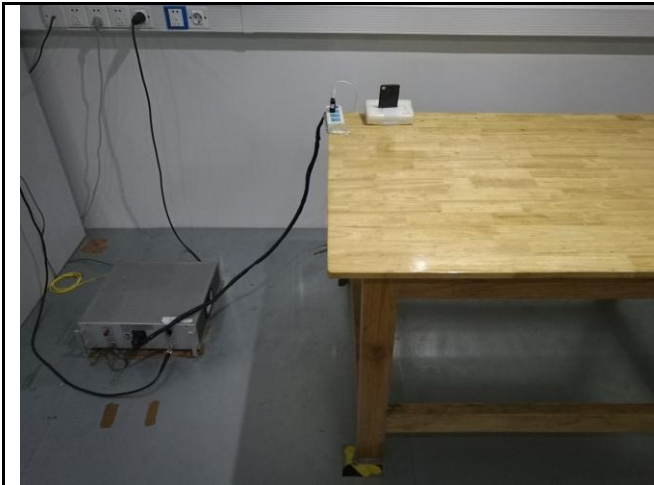
Conducted Emissions Test Setup Front View
