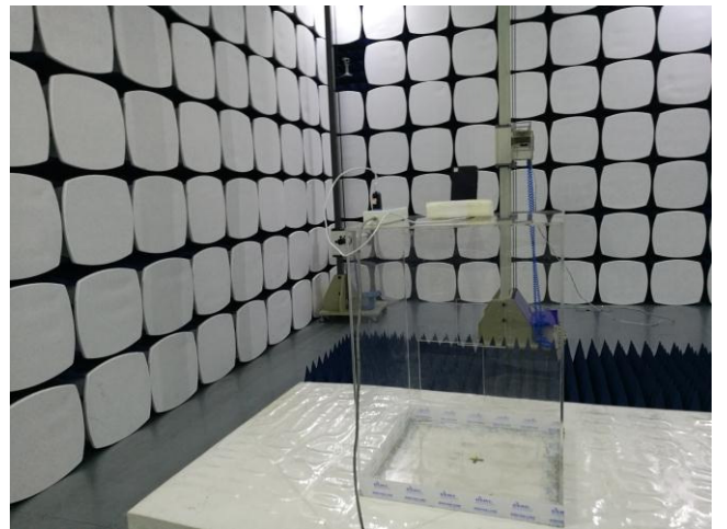
Radiated Spurious Emissions Test Setup Above 1GHz
