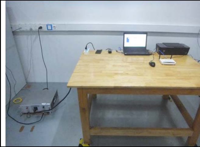
Conducted Emissions Test Setup – Front View
