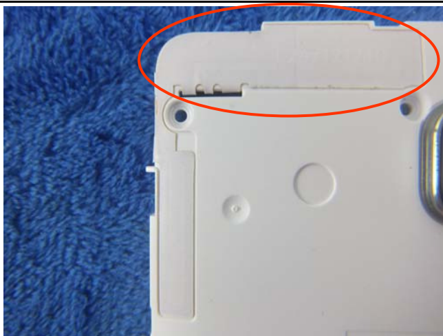
LTE - Antenna View
