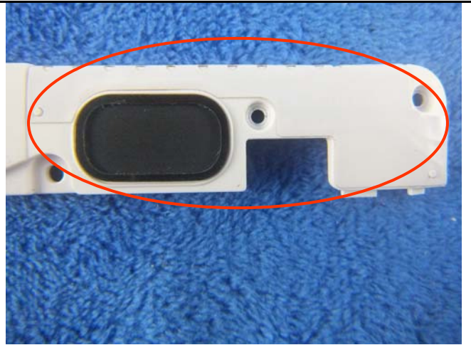
GSM/PCS/UMTS-FDD Antenna View
