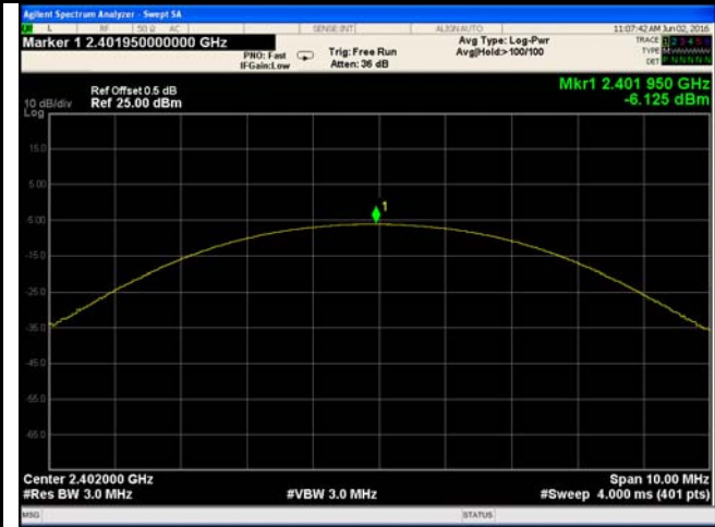
8DPSK Output power - Low CH 2402
