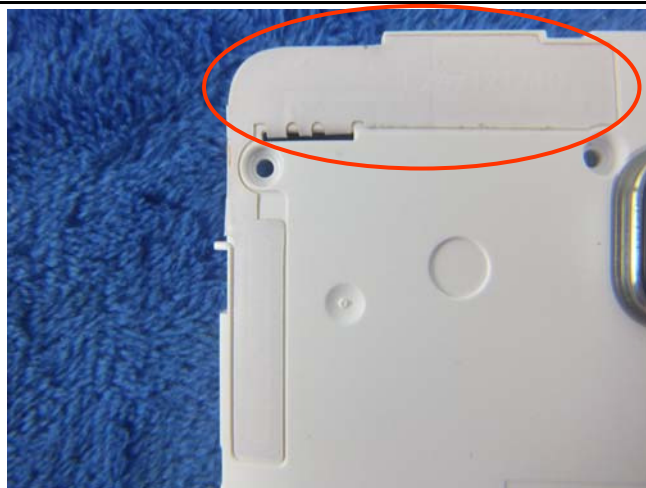
LTE - Antenna View
