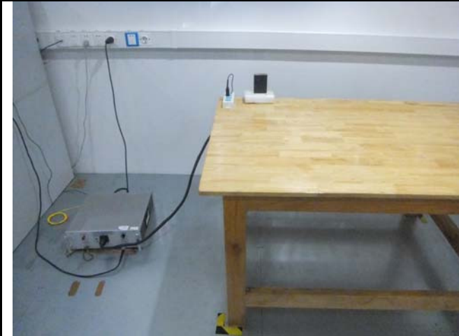
Conducted Emissions Test Setup Front View
