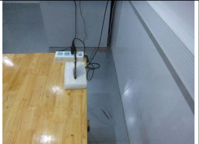
Conducted Emissions Test Setup Side View
